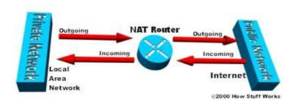
This is where NAT (RFC 1631) comes to the rescue. Basically, Network Address Translation allows a single device, such as a router, to act as agent between the Internet (or "public network") and a local (or "private") network. This means that only a single unique IP address is required to represent an entire group of computers to anything outside their network.
