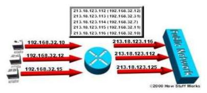
• Overloading A form of dynamic NAT that maps multiple unregistered IP addresses to a single registered IP address by using different ports. Known also as PAT (Port Address Translation), single address NAT or port–level multiplexed NAT.
